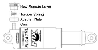
Fig. 1 Adapter Plate, Spring and Lever Installation
